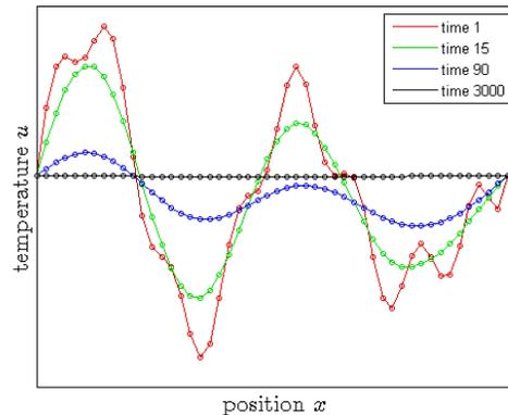
Figure 1: Temperature evolution along a rod at times  $t = 1, 15, 90, 3000$ ; for simplicity we assume the temperature is equal at both ends of the rod and remains constant.
